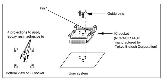
Figure 3 Location Setting of IC Socket
